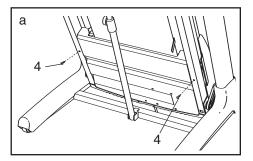
Lower the treadmill (see HOW TO LOWER THE TREADMILL FOR USE on page 24). Remove the four indicated 3/4" Screws (4), and remove the Hood (44).
